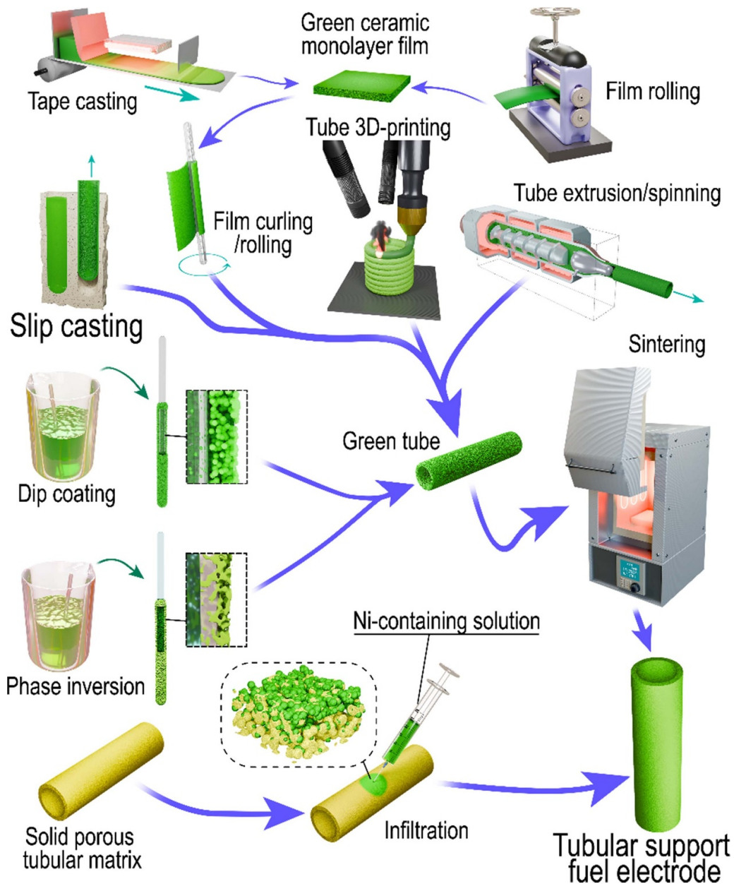
Figure 3. Various approaches to prepare protonic ceramic electrochemical support tubes.
