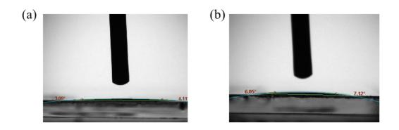
**Figure S3**. (a) contact angle of PeQD ink on PTAA substrate. (b) contact angle of PeQD ink with PB on PTAA substrate.
