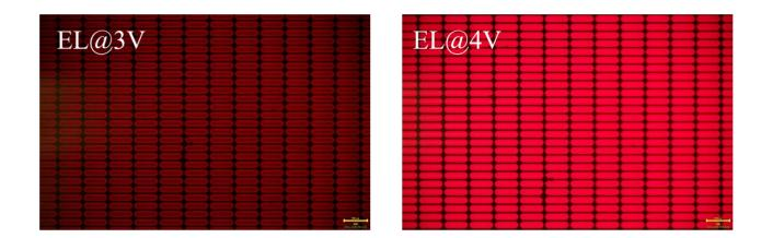
Figure S4. Light-on images of inkjet-printed matrix PeQD-LED with PB with a bias of 3V (left) and 4V (right) (scale bar: 200  $\mu$ m).
