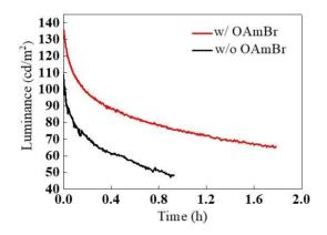
Figure S2. Lifetimes of the PeQD-LEDs with and without OAmBr.
