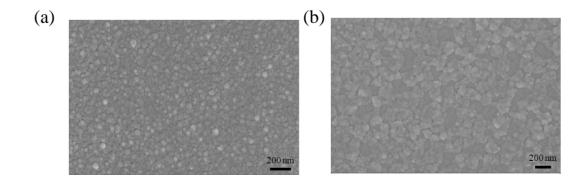
**Figure S5**. (a) SEM image of spin coated PeQD film on PTAA. (b) SEM image of inkjet-printed PeQD film on PTAA.
