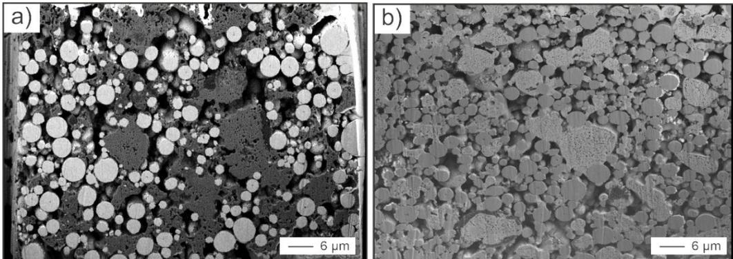
**Figure S4.** Cross-sectional FIB-SEM slice images of slurry-cast cathodes with (a) glassy SE (1.5Li<sub>2</sub>S-0.5P<sub>2</sub>S<sub>5</sub>-LiI) and (b) crystalline SE (Li<sub>6</sub>PS<sub>5</sub>Cl). Note that the cathode was not cold-pressed prior to the measurement. More pores within the SE particles are observed for the c-SE cell than the g-SE cell. Panel (a) shows a backscattered electron image and panel (b) is a secondary electron image.
