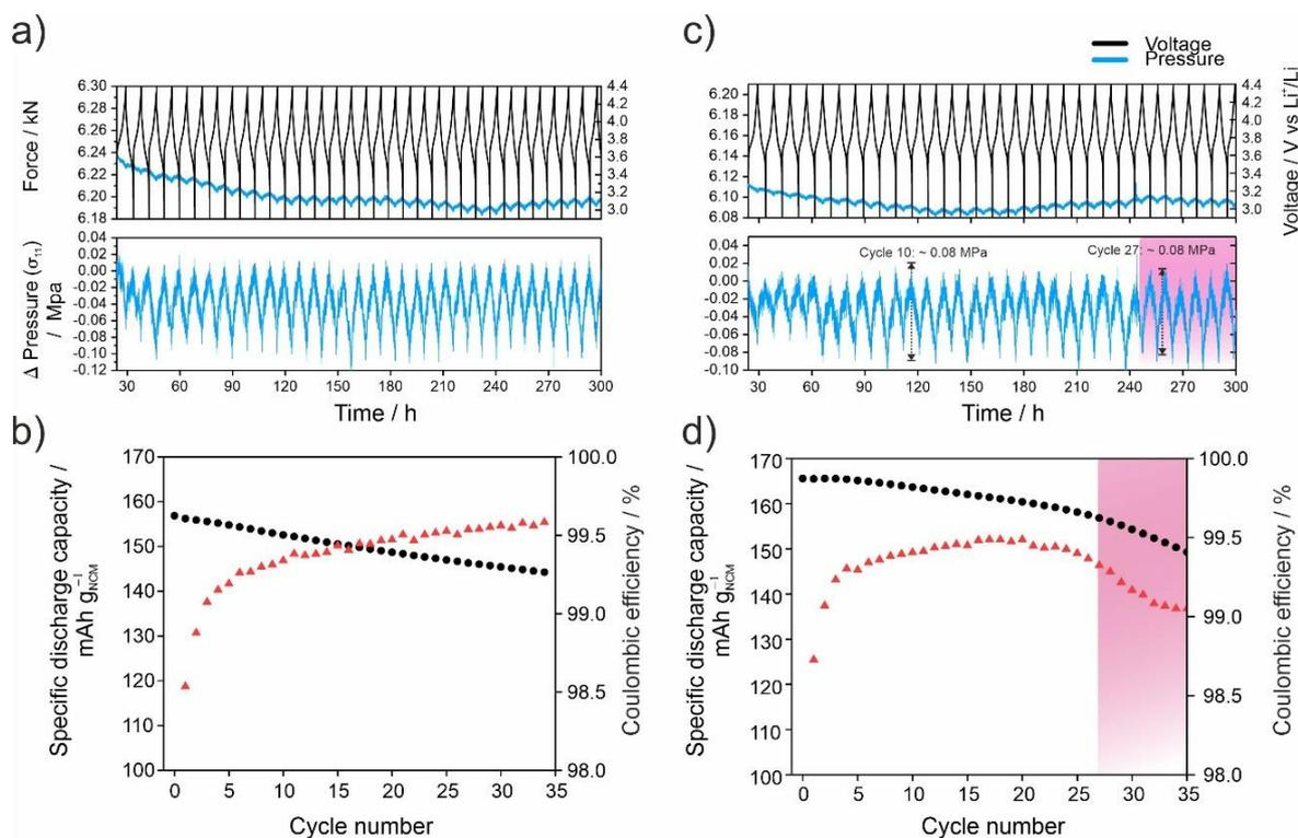
**Figure S6.** Force and pressure response during cycling of slurry-cast cathodes with (a) glassy SE ( $1.5\text{Li}_2\text{S}-0.5\text{P}_2\text{S}_5\text{-LiI}$ ) and (c) crystalline SE ( $\text{Li}_6\text{PS}_5\text{Cl}$ ) and (b, d) corresponding specific discharge capacities and Coulombic efficiencies over 35 cycles. SSB cells tested at  $45^\circ\text{C}$ , C/5, 2.9-4.4 V vs  $\text{Li}^+/\text{Li}$ .
