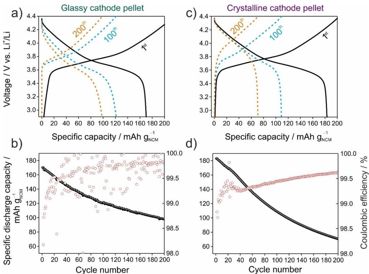
**Figure S1.** Representative 1<sup>st</sup>, 100<sup>th</sup>, and 200<sup>th</sup> cycle charge/discharge curves at a rate of C/5 and 45 °C of pelletized SSB cells with (a) glassy SE (1.5Li<sub>2</sub>S-0.5P<sub>2</sub>S<sub>5</sub>-LiI) and (c) crystalline SE (Li<sub>6</sub>PS<sub>5</sub>Cl) and (b, d) corresponding specific discharge capacities and Coulombic efficiencies over 200 cycles.
