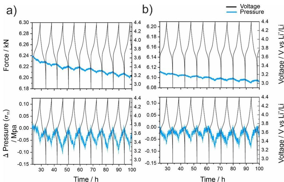
**Figure S5.** Raw data of the uniaxial force of slurry-cast cathodes with (a) glassy SE ( $1.5\text{Li}_2\text{S}-0.5\text{P}_2\text{S}_5\text{-LiI}$ ) and (b) crystalline SE ( $\text{Li}_6\text{PS}_5\text{Cl}$ ) recorded during cycling and the corresponding change in uniaxial stress ( $\sigma_{11}$ ) after baseline correction. SSB cells tested at  $45^\circ\text{C}$ , C/5, 2.9-4.4 V vs  $\text{Li}^+/\text{Li}$ .
