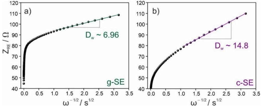
**Figure S3.** The real part of impedance data plotted versus the  $(\text{frequency})^{-1/2}$  and corresponding linear fit at low frequencies for (a) the g-SE cell and (b) the c-SE cell after 200 cycles at a rate of C/5 and 45 °C.
