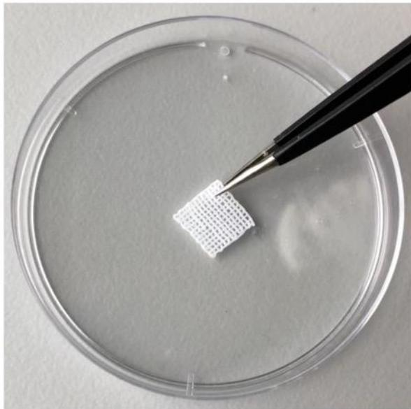
**Mov. S2.** The flexibility of the P34HB/PCL scaffold, which can be easily stretched, twisted, and rapidly returned to its original shape after removal of the external force.
