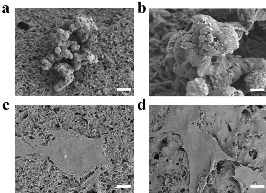
**Fig. S8.** SEM images of HUVECs (a, b) and BMSCs (c, d) on the surface of P34HB/PCL scaffolds. The scale bars are a) 50 μm, b) 10 μm, c) 50 μm, and d) 10μm, respectively.
