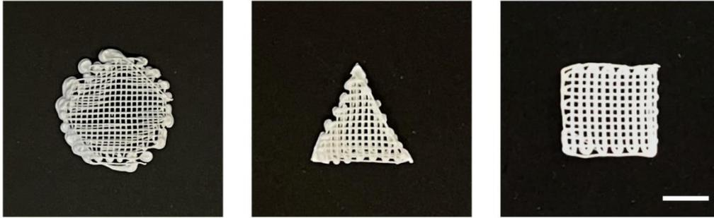
**Fig. S3.** Digital images of different shapes of the P34HB/PCL scaffolds were prepared by changing the array design. The scale bar is 10 mm.
