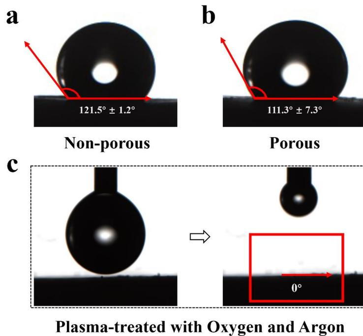
**Fig. S5.** The hydrophilicity of P34HB/PCL non-porous scaffolds (a), porous scaffolds (b) and plasma-treated scaffolds (c) evaluated by a water contact angle measuring instrument.
