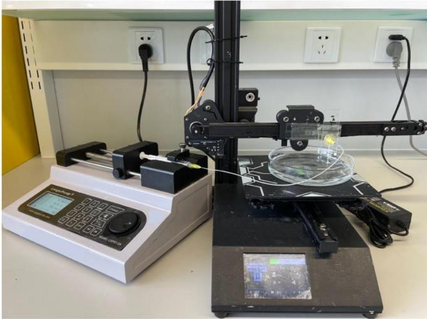
Fig. S1. Digital image of the microfluidic and 3D-printing device.
