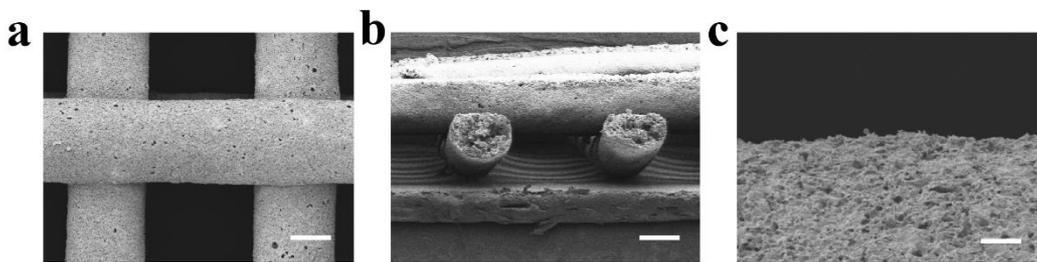
**Fig. S4.** SEM image of the P34HB/PCL scaffold. The scale bars are a) 150  $\mu\text{m}$ , b) 250  $\mu\text{m}$ , and c) 15  $\mu\text{m}$ , respectively.
