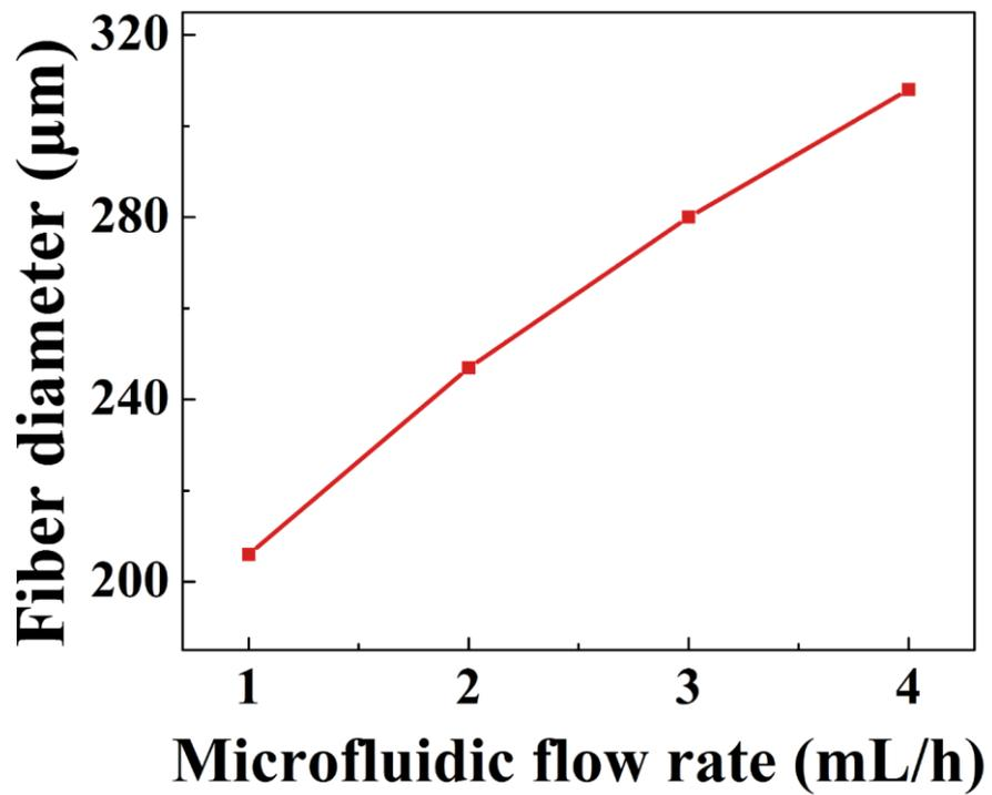
Fig. S2. Relationship between the P34HB/PCL microfiber diameter and the microfluidic flow rate.
