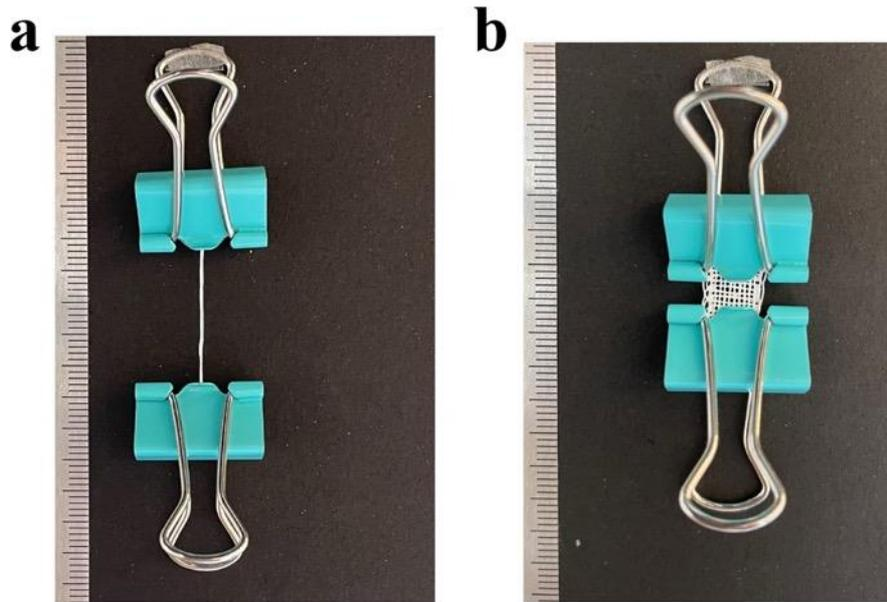
**Fig. S6.** Digital photographs showing the stretchability of the P34HB/PCL microfluidic fiber (a) and scaffold (b).
